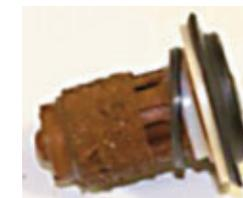
Clogged pressure regulator strainer on instant water heater.
